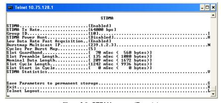
Figure 3-8 STDMA screen (Remote)
