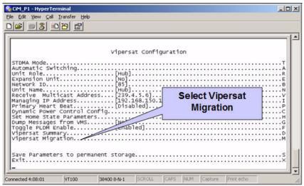
Figure D-22 Vipersat Configuration screen
