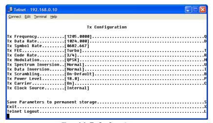
Figure 2-8 Tx Configuration screen
