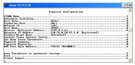
Figure 2-9 Vipersat Configuration screen (Hub)
