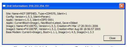
Figure D-16 Unit Information screen (Base Modem Image 1)
