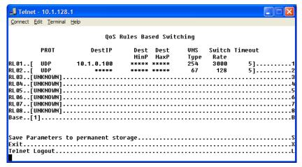
Figure 3-38 QoS Rules Based Switching screen
