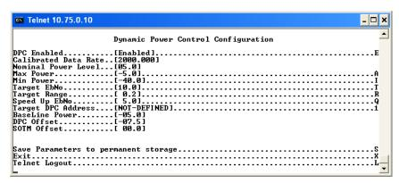
Figure 3-61 DPC Configuration screen (STDMA mode)
