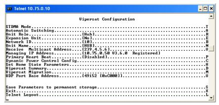
Figure 3-6 Vipersat Configuration screen (Hub)
