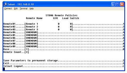
Figure 3-20 STDMA Remote Policies screen (GIR Hub)
